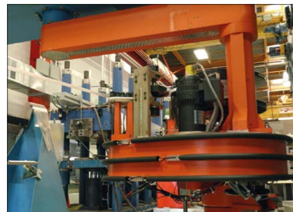
Fermilab's Giorgio Apollinari in the former assembly hall of the CDF experiment, where preparations for HL-LHC magnets are under way (top); flat Nb 3 Sn cables, coloured white after treatment with glass fibre to insulate each spire, are slowly fed from the coil winder to form prototype dipole magnets for the HL-LHC (middle and above).
