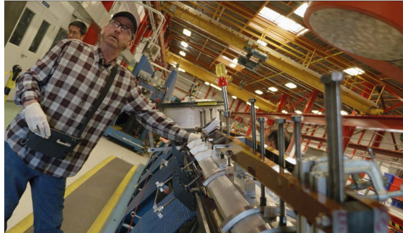
Superconducting niobium-tin cables being wound on the Spirex coil winder at Fermilab. (All image credits: J Ordan/CERN.)
